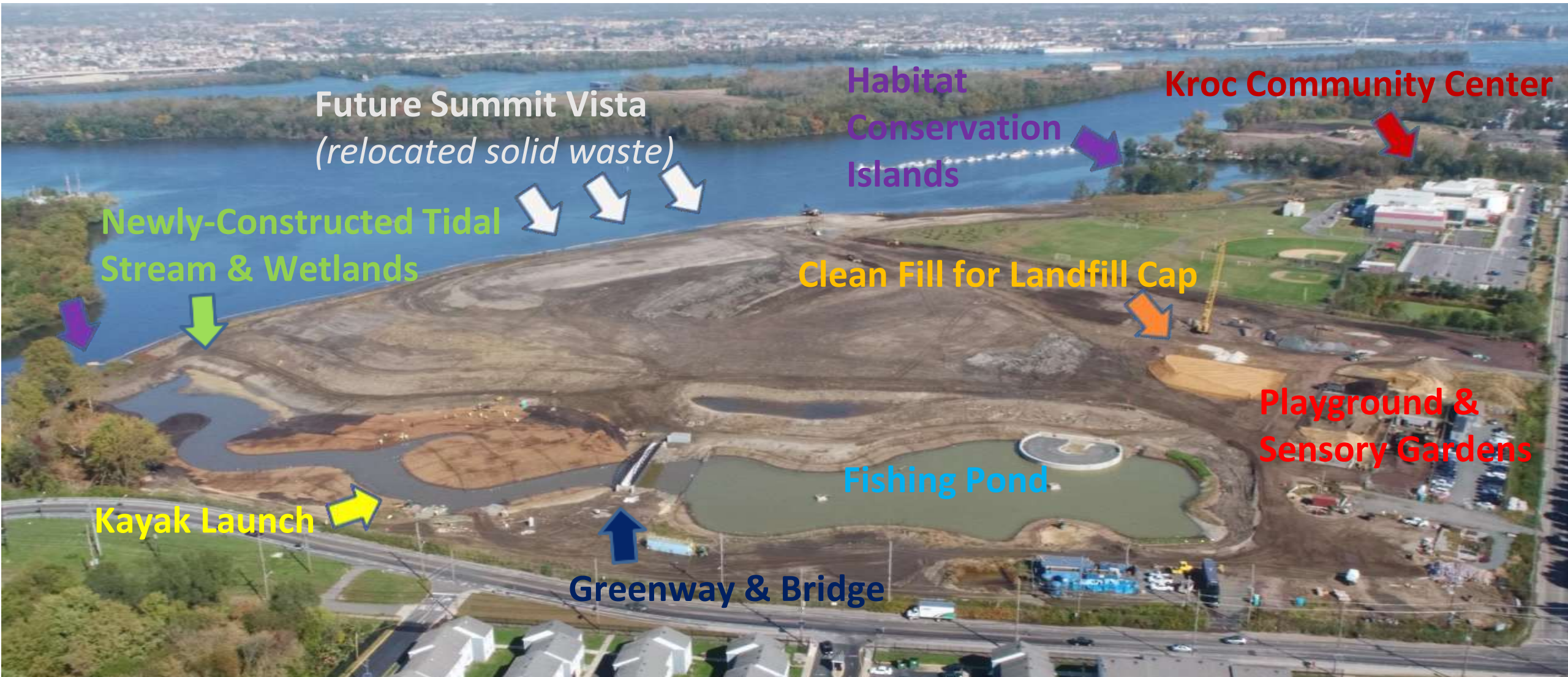
Aerial View toward north during remediation for Cramer Hill Waterfront Park (October, 2019), showing many of the resilient elements & community assets. Kroc Community Center is in the far upper right of aerial photo (courtesy of NJDEP Office of Natural Resource Restoration).
